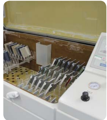
To conduct accelerated corrosion testing in the laboratory, a Q-Fog machine exposes panels to a cyclic environment of salt-laden fog, heat and humidity.
