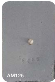
Test panels taken from an area of a test structure, not washed by rain, show minimal edge corrosion on ZINCALUME® steel AZ150 and almost no edge corrosion on ZINCALUME® steel AM125.
