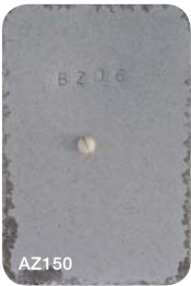
Test panels taken from an area of a test structure, not washed by rain, show minimal edge corrosion on ZINCALUME® steel AZ150 and almost no edge corrosion on ZINCALUME® steel AM125.
